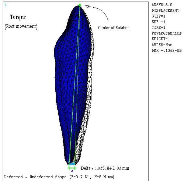
**Figure 2: simulation of torque movement**
